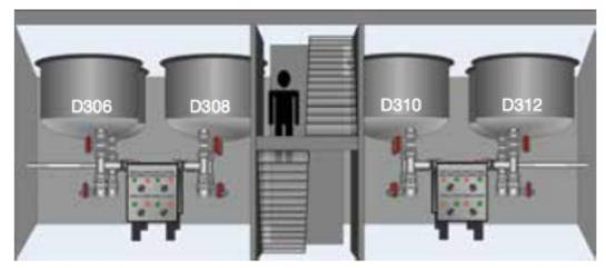
The operator instead, thinking he was at the right reactor and that the bottom valve wasn't functioning, overrode the interlock without consulting the reactor at the control panel. Once opened, VCM poured out and filled the building with liquid and vapor. The VCM vapors found an ignition source and several explosions occurred. The ensuing fire spread to the PVC warehouse and burned for hours, sending a plume of acrid smoke into the nearby community. **Causes**
